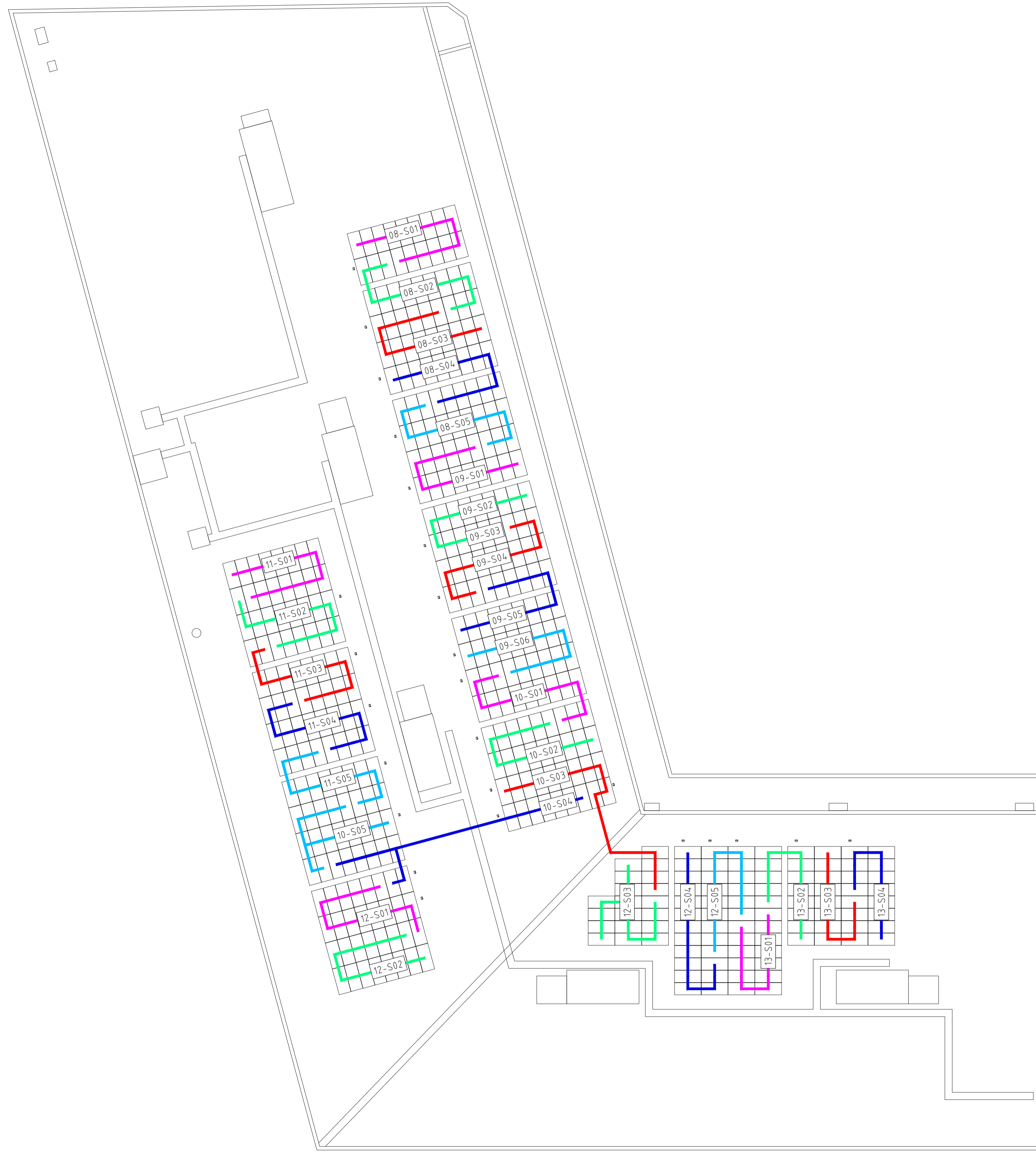
DC STRING LAYOUT (ROOF 2) SCALE 1:200
